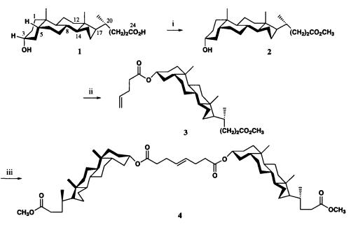
i) AcCl/MeOH; ii) 4-pentenoic acid, 2,6-dichlorobenzoyl chloride, Et<sub>3</sub>N, THF, reflux, 24 h; iii) Five mol % of 1,3-bis(2,4,6-trimethylphenyl)-2-imidazolidinylidene)(dichlorophenylmethylene)(tricyclohexylphosphene) ruthenium(IV) under nitrogen, CH<sub>2</sub>Cl<sub>2</sub>, reflux 6 h
